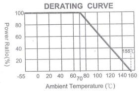
Power rating or current rating is in the case based on continuous full-load at ambient temperature of  $70^{\circ}$ C. For operation at ambient temperature in excess of  $70^{\circ}$ C, the load should be derated in accordance with figure of derating Curve.
